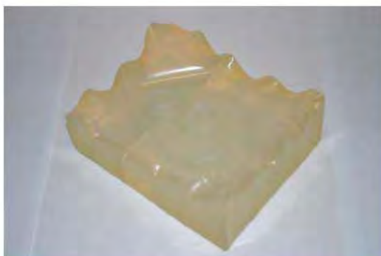
Obr.12 Silikónová forma zhotovená technológiou Vacuum Casting [8]
