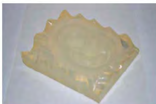
Obr.12 Silikónová forma zhotovená technológiou Vacuum Casting [8]
